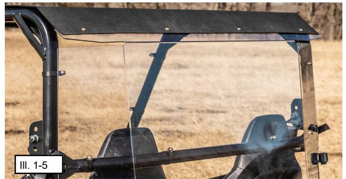
7. Assemble the roof to the top edge of the windshield and to the top edge of the back panel using (8) M5 x 16 mm Button Head Screws (Item 5), (8) Domed Shoulder Washers (Item 6) and (8) M5 Lock Nuts (Item 7). See Illustration 1-5 and 1-6.
