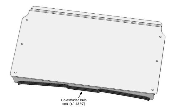
b) Install the windshield to the vehicle using supplied hardware (Item C). Adjust the position of the windshield and tighten. Caution: over tightening any hardware could cause irreversible damage to the windshield.
