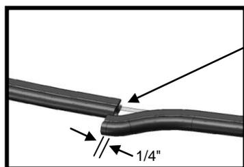
Co-extruded bulb seal starting/finishing point
