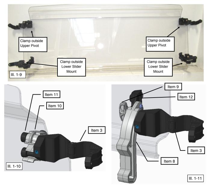
15. Ensure the clamps are open. With one person on the drivers side and one person on the passengers side, lift and position the Upper Windshield assembly onto the ROPS with the bottom edge contacting Foam Seal (Item 15) on the Lower Windshield assembly. See Illustration 1-12.
