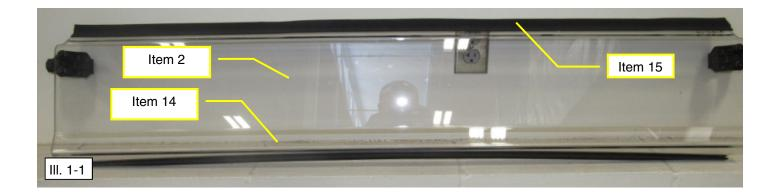
4. Assemble (1) Clamp (Item 3) on the drivers side of the Lower Windshield (Item 2) using (2) M6 x 18mm Button Heads (Item 4), (2) M6 Lock Washers (Item 5), and (2) Dome Shoulder Washers (Item 6). Do not tighten at this time to ease installation onto the vehicle. For proper fitment ensure "Kolpin" is facing outward on the clamps. Repeat for passenger's side. See Illustration 1-2.
