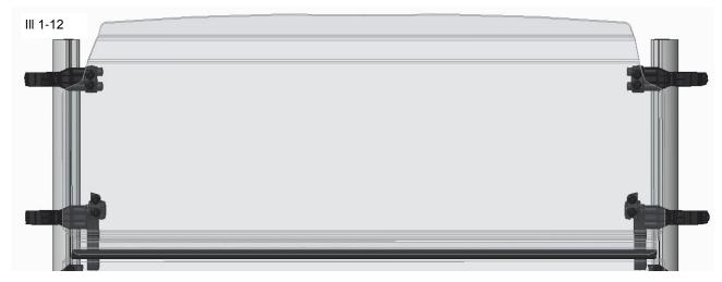
16. Loosely assemble (4) M6 x 14 Socket Head Cap Screws (Item 7) connecting the clamps (Item 3) around the ROPS. See Illustration 1-13 & 1-14.
