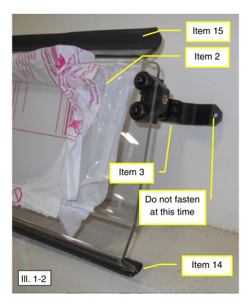
5. Take the Lower Windshield Assembly and position onto the ROPS and against the hood surface. Tighten to specification (2) M6 x 14mm Socket Head Cap Screws (Item 7) that secure (2) clamps around the ROPS. Then, tighten to specification (4) M6 x 18mm Button Heads (Item 4) and (4) M6 Lock Washers (Item 5) into (2) clamp assemblies to secure the clamps around the ROPS. See Illustration 1-3 and 1-4.
