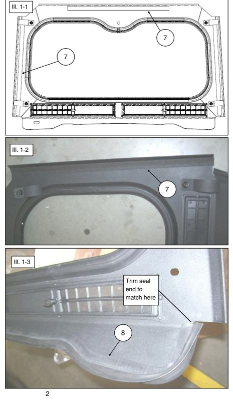
By firmly pressing with hand, install the bulb trim seal (item #8) onto the front lower surface of the glass windshield (item #1) as shown. Trim seal ends to match up with location as shown. (See illustrations 1-3 and 1-4). Note: The bulb trim seal has metal retainer strip, recommended cutting tool is metal shears/tin snips.
