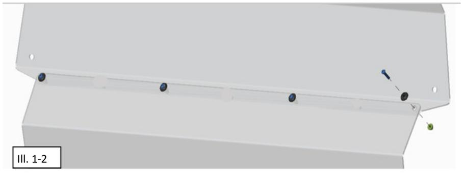
4. Assemble the Upper Windshield (Item 1) to the Lower Windshield (Item 2), using (4) M6 x 18mm Button Heads (Item 4), (4) Dome Shoulder Washers (Item 6), and (4) M6 Flange Locknuts (Item 8). See Illustration 1-2.
