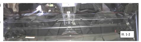
6. Install (3) clamps that secure the lower panel to the B pillar using (2) M6 x 18mm Button Heads (Item 4), (2) M6 Lock Washers (Item 5), and (2) Domed Shoulder Washer (Item 6). See Illustration 1-3, 1-4, and 1-5.
