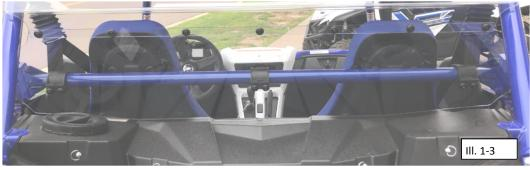
Insert (1) Clamp Spacer (Item 9) into each Clamp and secure the clamp to the ROPS using (1) M6 x 18mm Button Head (Item 4) and (1) Lock Washer (Item 5).
