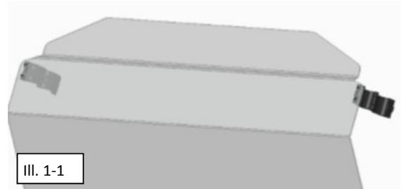
4. With one person on the drivers side and one person on the passenger's side, lift and position the windshield assembly onto the ROPS. Loosely assemble (2) M6 x 18 Button Heads (Item 4) and (2) Lock Washers (Item 5) connecting the male & female clamp parts around the ROPS.
