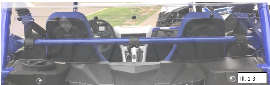
7. Insert (1) Clamp Spacer (Item 9) into each Clamp and secure the clamp to the ROPS using (1) M6 x 18mm Button Head (Item 4) and (1) Lock Washer (Item 5). See Illustration 1-3, 1-4, and 1-5.
