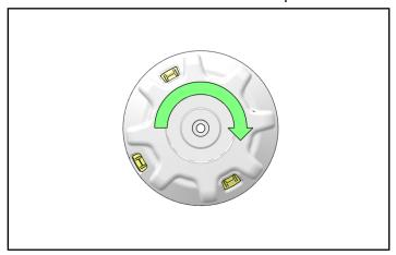
To shift into low, rotate the gear shifting knob counter-clockwise until the "L" marking shows thru the cutout window on the shift knob. See photo below.
