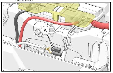
Route the remaining black negative (-) wire (2D) on the control box ② to the negative (-) terminal of the battery. DO NOT CONNECT at this time
