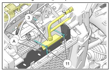
b. Route orange and black power wires from wireless receiver to the battery compartment area. Attach cables to chassis/frame at various locations using supplied cable ties to ensure the cables stay clear of any moving parts. sharp edges and/or hot surfaces. DO NOT connect at this time.
