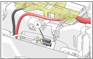
Route the remaining black negative (-) wire (3B) on the control box ③ to the negative (-) terminal of the battery. DO NOT CONNECT at this time
