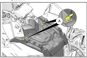
b. Lift the rear of the rack upwards and remove front rack.
