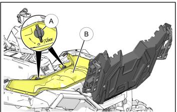
c. Lift the protective rubber battery cover © to gain access to the battery terminals.
