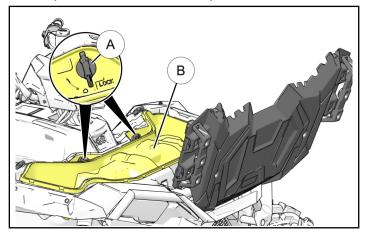
b. Close front rack/storage bin cover ① and secure using latches ①.
