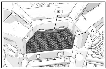
b. Next, remove the four fasteners that secure the front fascia to the vehicle and remove front fascia.
