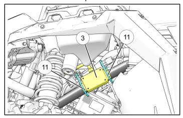
Route orange and black power wires from wireless receiver to the battery compartment area. Attach cables to chassis/frame at various locations using supplied cable ties to ensure the cables stay clear of any moving parts, sharp edges and/or hot surfaces. DO NOT connect at this time.
