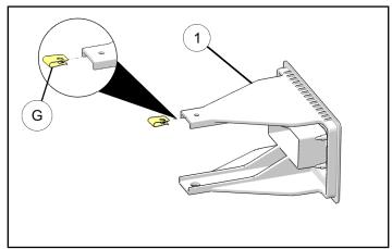
7. Ensure "POLARIS" text on front face of intercom mount ① is oriented properly, then hook lower tab and rotate mount up to lock into dash panel.
