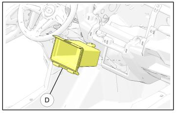
6. Remove nut clip (G) from upper rear flange of storage compartment (D), then reinstall nut clip on upper rear flange of intercom mount ① as shown. Ensure proper orientation of nut clip.
