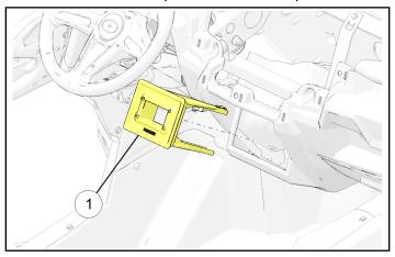
8. Install retained screw (E) to secure bracket (F) to upper rear flange of storage compartment ① as shown.
