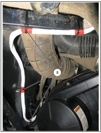
d. Route gain control harness ⑤ inboard of air intake tube, up through hole in vehicle bed as shown, then to subwoofer ①.
