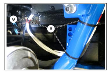
b. After exiting center console, route gain control harness ⑤ outboard to vehicle frame, up and around air intake tube, then rearward along frame as shown.
