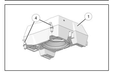
Ensure both expansion anchors (4) are unlocked, then insert two mounting brackets (1) attached to front of subwoofer (1) into corresponding mounting slots in vehicle bed.
