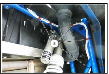
c. Route gain control harness ⑤ from wheel well up through gap between base of ROPS C-pillar (4 Seat: D-Pillar) and body panel as shown, then to subwoofer ①.
