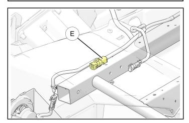
6. Install battery connection cable assembly 8.
