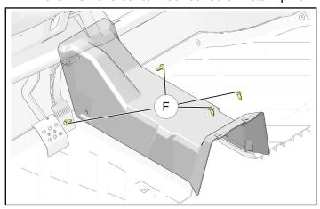
b. Starting from center floor console, route front end of cable assembly ® (identified by red terminal cap) forward along main vehicle harness, up forward side of firewall, across and up through under-hood liner, then to terminal block. Secure cable assembly to firewall using three fir tree clips © as shown.
