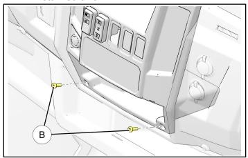
Carefully pull control panel away from main dash panel. Label electrical harnesses as required, then disconnect harnesses and remove panel. c. Remove switches from existing control panel.
