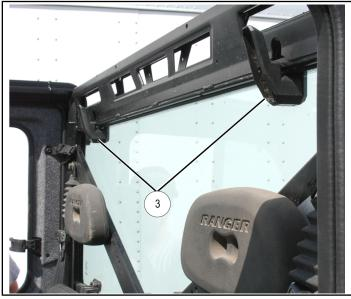
5. To remove, rotate handles ③ counterclockwise to unlocked position, tip upper edge of panel slightly rearward, then then lift panel brackets ⑥ from vehicle frame.
