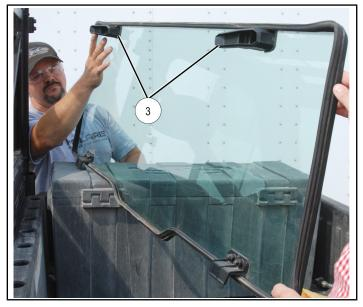
Lower panel brackets (6) into vehicle frame as shown, then tip upper edge of panel forward into ROPs. Ensure panel is centered from right to left.
