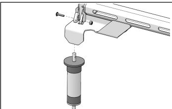
Insert box rails ② into vehicle so that expansion anchors ① fully recede into vehicle receptacles as shown, then depress upper cams to lock in place. If installation is loose, remove box rails from vehicle, tighten nuts at base of expansion anchors, and reinstall.
