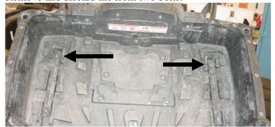
3. Install the brushguard mounts to the box frame as shown. Secure the front using the 5/16-18 x 2.50" machine screws included with this kit. Use the nylock nuts removed in step 1. Leave the nylock nuts finger tight only at this time.
