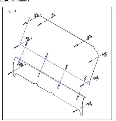
Position windshield onto machine. Place the eight clamps around the perimeter of the cab frame. Now install the windshield to the clamps using the remaining 8 screws, fender washers, and flange nuts as shown.
