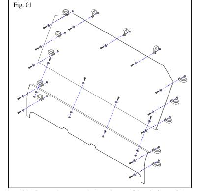
Position windshield onto machine. Place the thirteen clamps around the perimeter of the cab frame. Now install the windshield to the clamps using the remaining 13 screws, fender washers, and flange nuts as shown.
