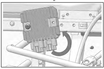
5. Use hole on regulator as a template and mark hole with marking tool.
