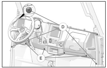
2. Secure steering grommet to dash with retained star washers ©.
