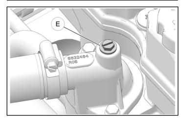
13. Tighten screw after air has been released. Torque to specification.
