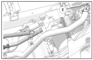
4. Tighten screw after air has been released. Torque to specification.
