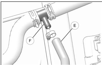
5. Connect top coolant hose  $\ \ \ \$  from heater to T-fitting  $\ \ \ \$  . Secure with hose clamp  $\ \ \ \$  . Torque to specification.
