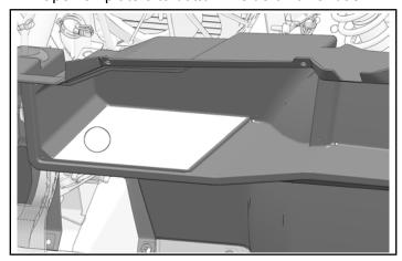
2. Drill hole through bottom of dash.
