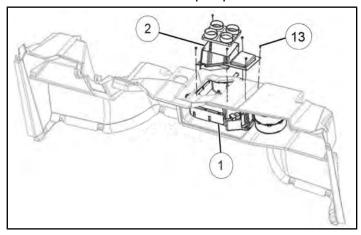
5. Install rubber bushings onto heater bolts.
