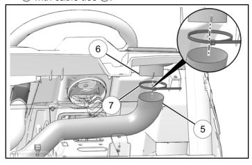
3. Secure short duct ④ to passenger side vent assembly ⑥ with cable ties ⑦.
