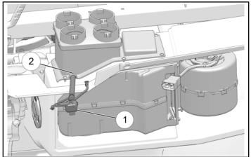
9. Install heater cap ② over dash cutout. Tighten screws ③ until fully seated.
