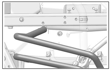
8. Inspect mounting screws for damage. If damaged, replace with new Torx Truss Head screw size M6 x 1.0 x 45
