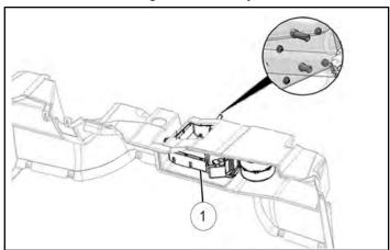
8. Thread electrical connections ① through top hole on lower dash and molded opening on heater cap
