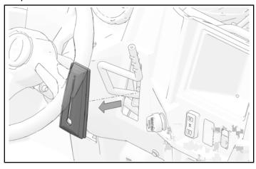
3. Remove and retain four push nuts © to detach steering boot from main dash panel.
