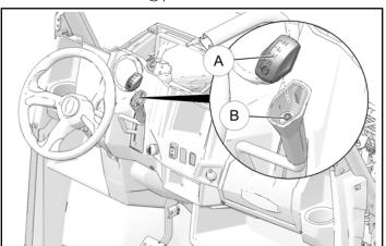
2. Remove and retain shift rod boot from main dash panel.
