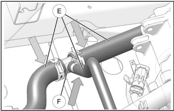
4. Remove small coolant hose **(E)** from T-fitting **(F)**. Retain hose clamp for future use.
