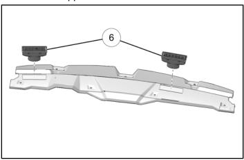
2. Insert vent assembly **(6)** into vent cutouts on main dash. Set main dash aside.
