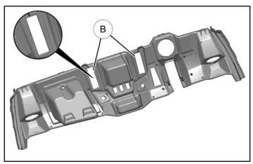
3. Cut out back of heater control panel location ©. Cut molded plastic compartment off, leaving 0.5 inch of molded plastic still attached to backside of main dash.
