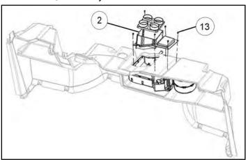
From inside vehicle, attach long duct ⑤ to back left position on heater cap ②. Secure with cable tie ⑦.
