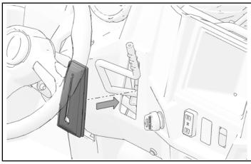
4. Reinstall shift rod handle. Secure shift rod handle to shift rod with retained screw (B). Tighten screw until fully seated. Carefully snap shift rod cap (A) onto shift rod handle.
