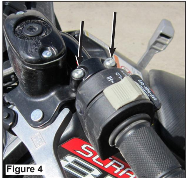
6. Remove clamp and install left hand handguard mount, reusing the screws removed in Step 5.
