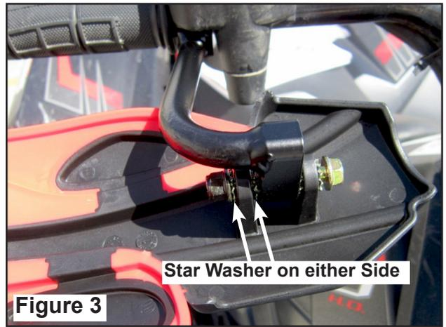
5. Remove the two screws from the top of the brake master cylinder clamp using a T30 Torx driver. Save screws for reassembly.
