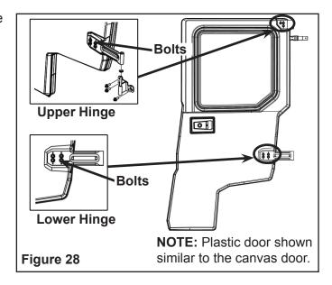
35. Rotate door out 90° and tighten top two bolts on the upper hinge bracket. Torque to 17 ft. lbs. (23 Nm). Figure 29.
