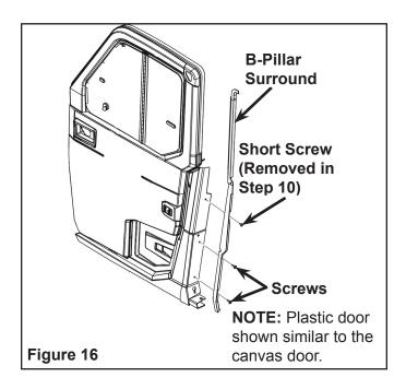
20. Mount the surround (PN 5450560 RH; 5450559 LH) on the B-pillar using three screws (PN 7519650) with Torx driver. Torque to 8 ft. lbs. (10.8 Nm). Figure 17.
