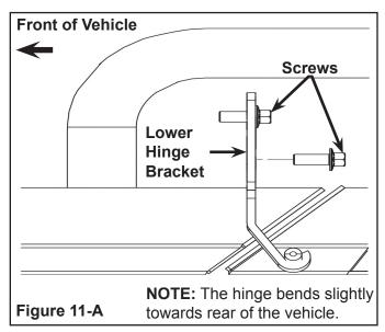
13. Install the C-pillar lower hinge bracket (PN 1018773 RH; 1018772 LH) using three screws (PN 7517838) in the existing holes on the vehicle with a 13 mm socket wrench. Torque to 17 ft. lbs. (23 Nm). Figure 12.
