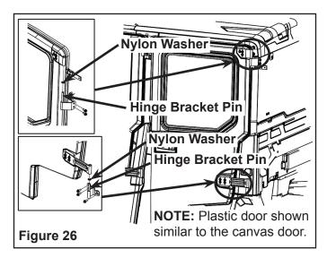
33. Loosen the upper and lower hinge brackets as necessary for proper door alignment. Use a 13 mm socket wrench. Align door using outside edge of door and ROPS frame to determine best fit. In order to maintain clearance to hinge for front doors, slide rear door slightly rearward in ROPS frame before tightening hinges. Figure 27.
