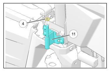
f. Reinstall B-pillar cover ® over lower hinge 11 using retained screws © and push darts D.
