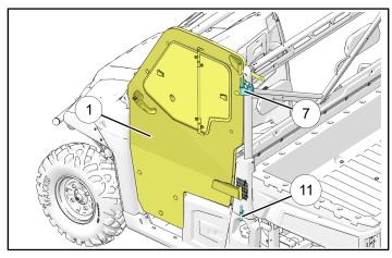
c. Close and center door in ROPS by pushing door inward and upward.
