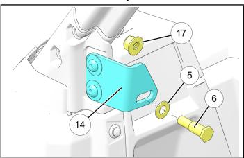
c. Open door latch (to properly position pawl), then slowly close door and observe engagement of striker pin 6 into door latch.
