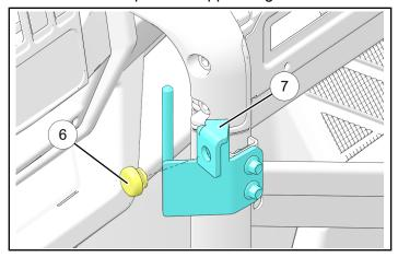
c. Install nylon washer 4 to upper hinge ①.
