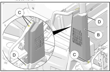
c. Cut slot in B-pillar cover ® at marked location €.
