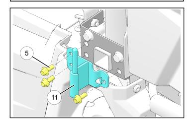
e. Install nylon washer 4 to lower hinge 11.
