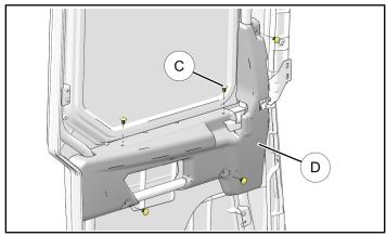
4. Install door liner ① using eight push darts ③ as shown. Do not install push dart in upper rear corner of door.
