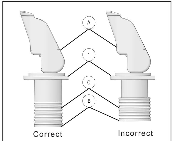
If the anchor tension is inadequate when securing the accessory to the ATV (in case of a heavier accessory), tighten the M6 shaft one turn at a time.
