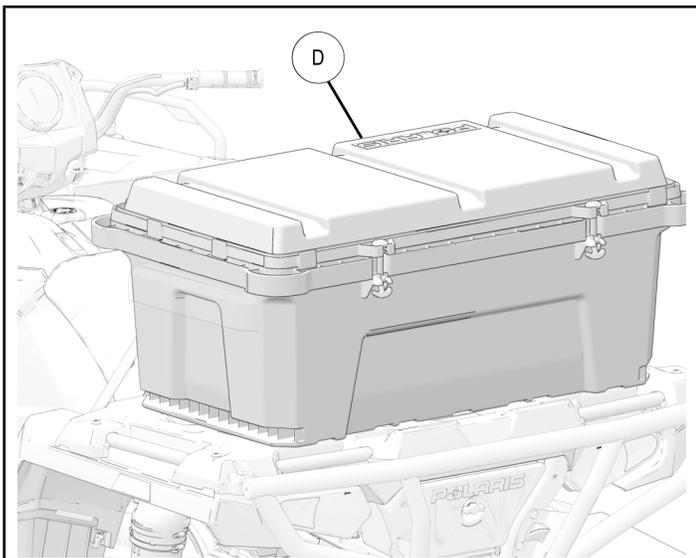
4. Insert the bracket (1) with lock and ride (2) to the storage box (D) grooves on both sides as shown.
