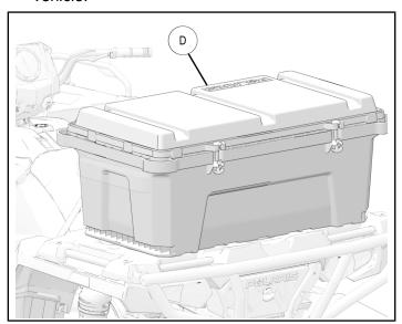
4. Insert the bracket ① with lock and ride ② to the storage box (D) grooves on both sides as shown.
