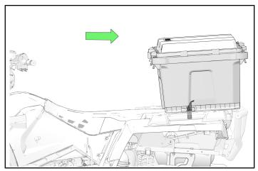
5. Secure the storage box to the vehicle by lock and rides on both sides.
