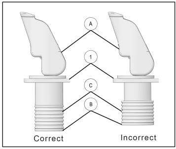
If the anchor tension is inadequate when securing the accessory to the ATV (in case of a heavier accessory), tighten the M6 shaft one turn at a time.
