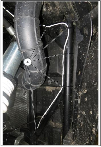
c. Route light harness across to vehicle centerline and forward into center console as shown, then to electrical box ①.
