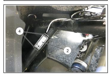
b. Route light harness up and across frame to vehicle centerline, then down towards main vehicle harness as shown.
