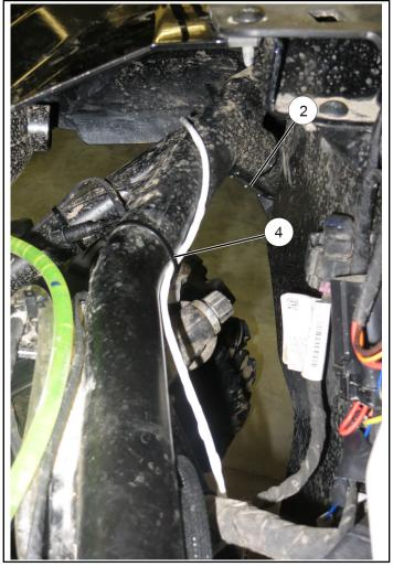
c. Route light harness down along main vehicle harness into center console as shown, then rearward to electrical box ①.
