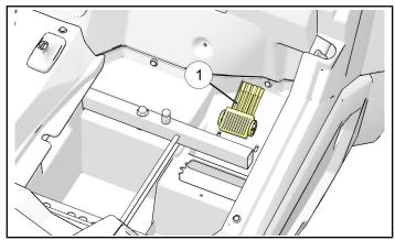
b. Route switch and power wires forward through center console, along main vehicle harness, to upper instrument panel compartment.
