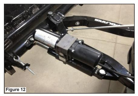
23. Connect the Angle cylinder to the plow control harness, turn the key to the ON position and test for proper operation.
