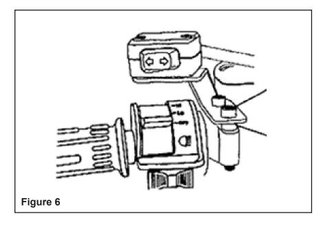
11. Locate the winch control switch, spacers and mounting nuts from the winch hardware kit and assemble these items. Figure 7. Tighten the switch retaining nuts until snug. If the winch switch in your kit was mounted on top of the left hand control, you will need to remount the winch switch. Figure 7.
