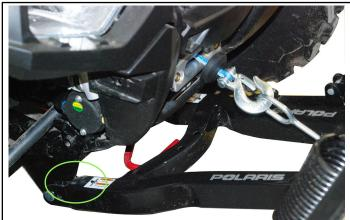
9. Press the locking handle (6) down to lock the plow in place on the ATV frame.
