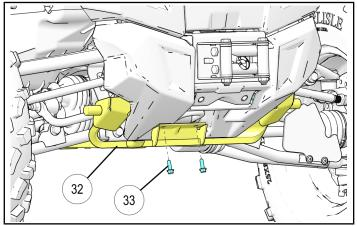
Fully tighten all hardware starting by front lower screws 3, then rear screws 5, and finally front side screws 1.
