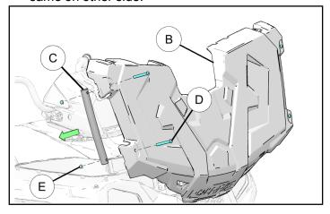
5. Using drill bit, drill two holes into the box cover (B) through existing indents (marked in red) (F).
