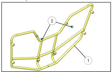
7. Mount the rack assembly ① onto the front box cover (B) by aligning holes as shown. Install two screws ③ from bottom into the rack assembly through the support bar (C). Don't tighten screws at this time.
