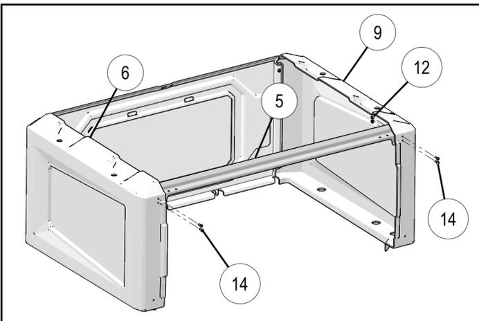
4. Insert four large LOCK & RIDE® expansion anchors ① in LH and RH side panels ⑥ ⑨ as shown.
