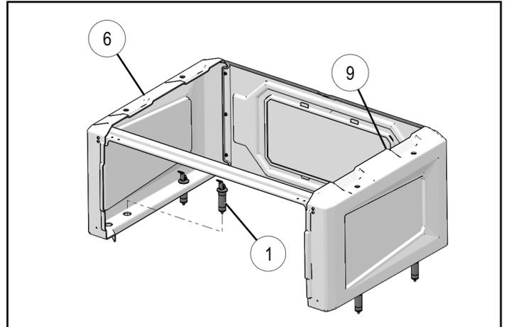
5. Install bed box assembly to vehicle until expansion anchors ① are fully seated, then depress upper cams to lock in place. If installation is loose, release affected cam lock, tighten nut at base of expansion anchor, and re-engage cam lock.
