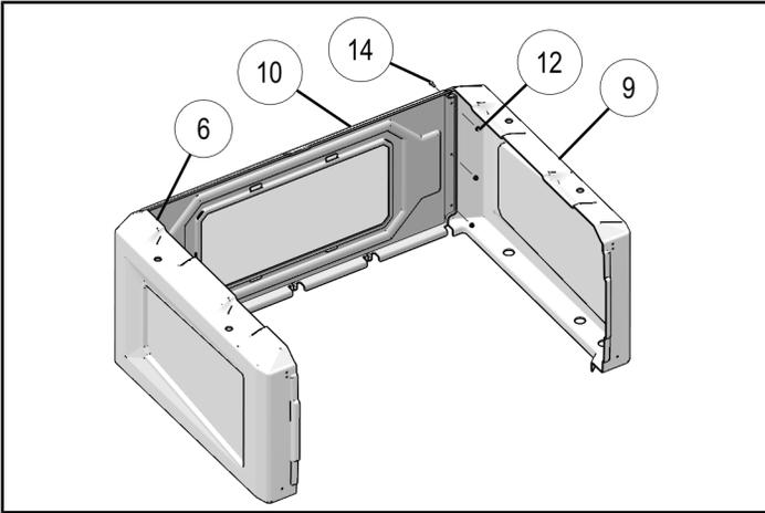
3. Install rear support bracket ⑤ to side panels ⑥ ⑨ using two screws ⑭ and nuts ⑫ per side as shown.
