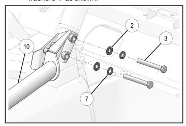
b. Loosely install support <sup>®</sup> at front attach point using M8 bolts <sup>®</sup> and nuts <sup>®</sup> as shown.
