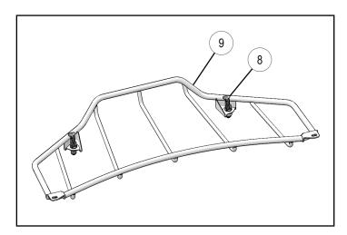
8. Loosely install left hook <sup>(5)</sup> to removable rack <sup>(9)</sup> using screws <sup>(1)</sup>, lock washers <sup>(7)</sup>, and flat washers <sup>(2)</sup> as shown.
