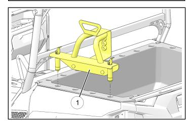
Install spare tire/wheel (sold separately) to mount frame ① using handle ② as shown. Three mounting hole options are provided: use hole which allows tire to rest on vehicle bed.
