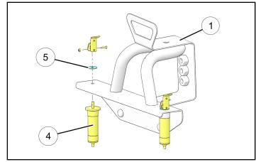
4. Ensure all expansion anchors ④ are unlocked, then install mount frame ① into bed until anchors are fully seated as shown. Depress levers to lock in place.
