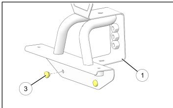
Install two LOCK & RIDE<sup>®</sup> expansion anchors ④ to mount frame ① per anchor kit instructions EXCEPT as follows: Insert washer ⑤ between lever and frame as shown.
