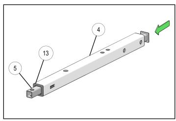
4. Insert cap (10) on upper end of tube (5) as shown. Ensure cap is fully seated so screw holes are aligned.
