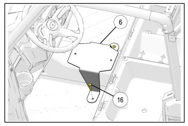
10. Install gun mount assembly to floor bracket ② ⑥ by inserting floor bracket studs ⑪ through fastener holes in base plate ③ as shown. Secure with nuts ⑫.
