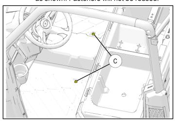
ii. Install floor bracket (6) using two screws (16) as shown.
