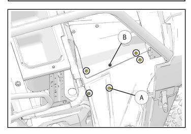
ii. Install floor bracket ② using two screws ⑯ in LH side of bracket and three screws ⑮ in RH side of bracket as shown.
