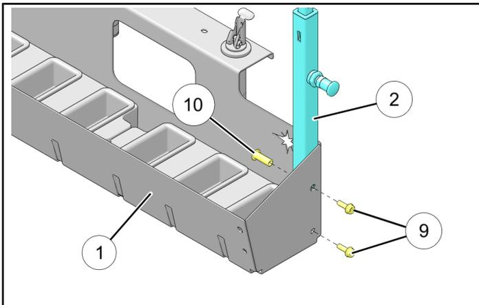
For installation to forward bed wall install clamp support in angled position:
