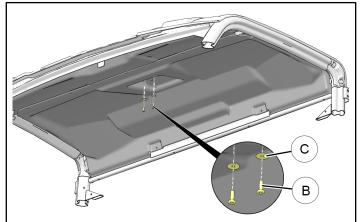
d. Carefully pull LH and RH edges of liner from between ROPS and roof seal, then remove rear edge of liner from roof support channel (D).
