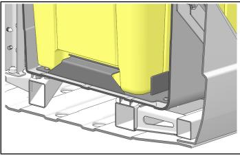
e. Secure front of subwoofer ① using screw ③ through drilled hole. Torque to specification.
