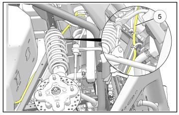
e. Route main harness ⑤ rearward until intake duct curves beneath battery. Route harness up and rearward along LH (driver) side of fuse box, then towards RH (passenger) side of vehicle along rear of battery.
