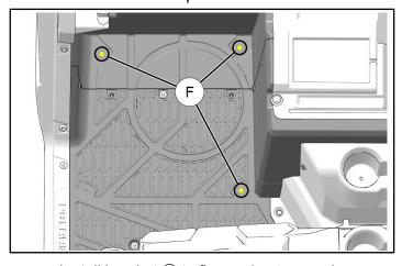
c. Install bracket 4 to floor using two each screws 2 and 3. Torque to specification.
