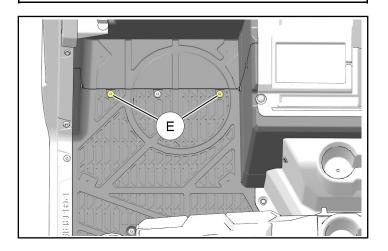
b. Drill 1/8 inch (3 mm) holes at three indented marks ①. Only drill deep enough to penetrate floor surface and enter pre-drilled bosses on underside of floor panels.
