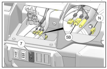
f. Reaching through cupholder cutout, join bass control connector ® to connector 5B on harness ⑤ (identified as REMOTE BASS).
