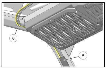
c. After harness exits lower end of conduit, route connectors 6A and 6B down through opening between base of A-pillar and upper dash panel, then inboard along dash support bracket towards cupholder opening.
