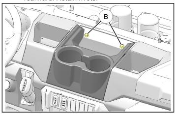
d. Remove four push pin rivets © from each side of center floor console, and two push pin rivets
