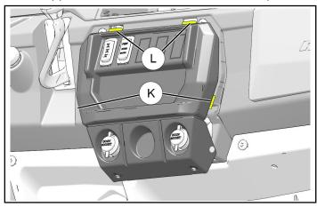
c. Label and disconnect electrical harnesses from switches, sockets, or other devices from control panel.
