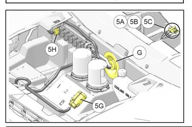
Drill out one accessory plug (1/4 inch / 6 mm) on under-hood liner, just forward of air intake ducts, then install relay/fuse block 5G using attached fir tree clip.
