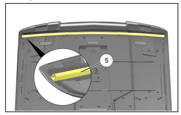
8. Peel adhesive backing from rear seal (3), then apply seal to rear edge of roof panel, aligning punched holes in seal with fastener standoffs in panel. Press seal firmly into place.
