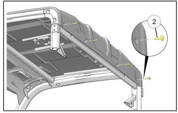
14. Torque screws 2 and 4 to specification.
