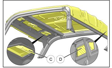
12. Secure front right corner of roof panel to ROPS using screw ④. Repeat for front left corner.
