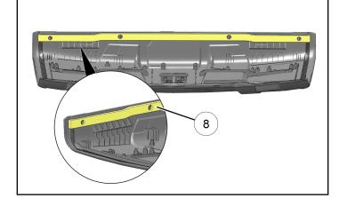
Peel adhesive backing from side seal ①, then apply seal to roof panel on outboard side of channel wall <sup>®</sup>. Trim side seal as required to fit between front seal <sup>⑤</sup> and rear seal <sup>®</sup>. Press seal firmly into place. Repeat for opposite side.
