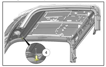
13. Secure rear edge of roof panel to ROPS using four screws ②.
