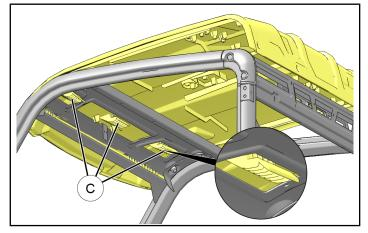
11. Slide roof panel rearward until hooks © lock into ROPS visor, then press rear of roof panel down until two tabs <sup>(1)</sup> snap into B-pillar cross-member.
