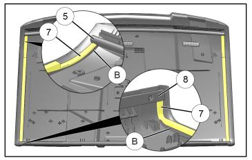
10. Lay roof panel ① on top of ROPS, inserting three hooks ① through openings in ROPS visor.
