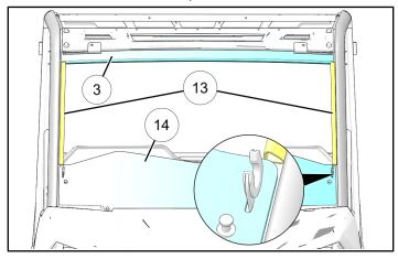
b. Position upper windshield ① as shown, then insert into hinge assemblies.
