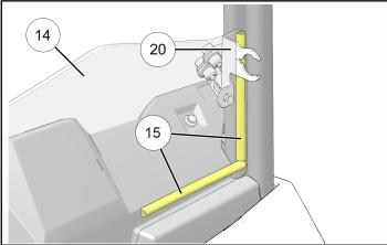
c. Peel off backing and apply **narrow** D-seal (5) to upper dash and A-pillars as previously shown, ensuring lower and side edges of windshield (4) will adequately contact D-seal as noted in previous step. Also ensure outboard end of horizontal D-seal is secured to A-pillar. Cut/trim seal as required. Repeat for opposite side.
