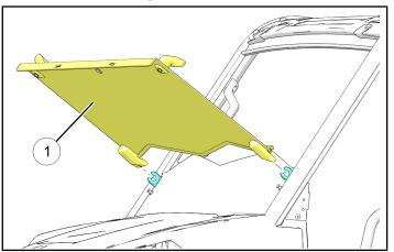
c. Tip upper windshield ① up as shown, then rotate both handles 1/4 turn to lock windshield to A-pillars. Adjust brackets ② and ② as required to ensure windshield is centered in ROPS opening.
