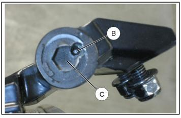
b. Rotate hinge pin eccentric cam © either direction as required. Repeat for opposite side hinge.
