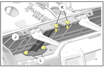
17. Install backing bracket (1) using two retained upper screws (1) and two new lower screws (2). Tighten screws.
