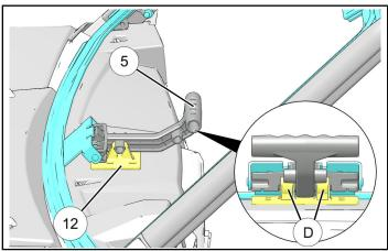
9. Pull handle (5) rearward to slightly compress windshield seal. While pulling handle, use handle base (12) as template to mark four holes (F) in upper dash panel.
