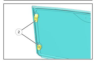
3. Place windshield ① into ROPS, then turn all four handles ② to locked position (perpendicular to sides of windshield).
