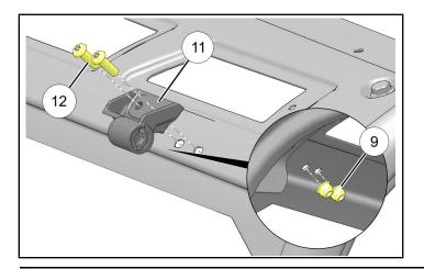
4. Using two people, lift windshield ① into position, sliding LH windshield side hinge ⓐ into vehicle side hinge ⑪ until ball end of hinge pin clicks into bushing.
