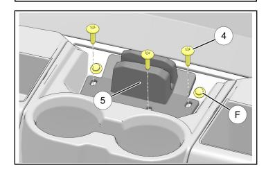
16. Close windshield and lock handle into base ⑤. Ensure windshield seal is adequately compressed and windshield opens/closes properly. Adjust as required.
