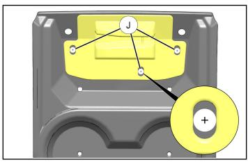
14. Drill 9/32 inch (7 mm) holes through cupholder at marked locations ①.
