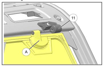
5. Assemble RH vehicle side hinge ① to windshield side hinge ③ until ball end of hinge pin clicks into bushing.
