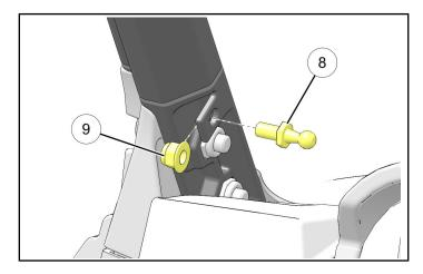
3. Install LH vehicle side hinge (1) to ROPS visor using two each screws (2) and nuts (9). Do not tighten nuts at this time.
