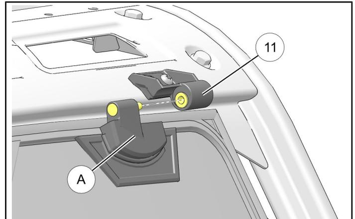
5. Assemble RH vehicle-side hinge (11) to windshield-side hinge (B) by sliding pin into bushing.
