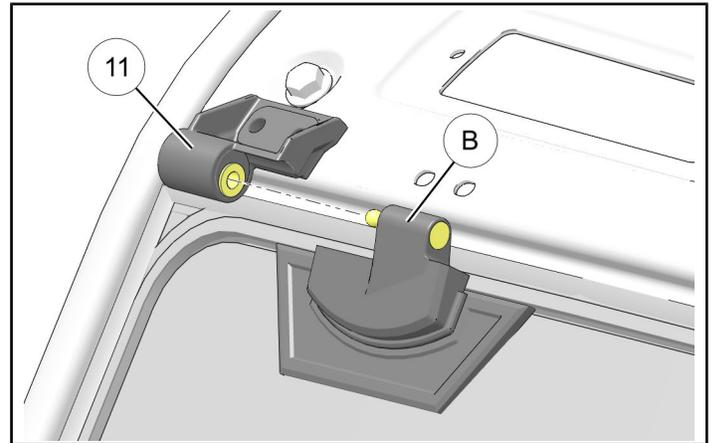
6. Install RH vehicle-side hinge (11) to ROPS visor using two each screws (12) and nuts (9). Tighten all four (LH and RH) hinge nuts.
