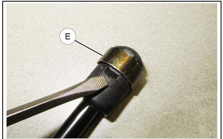
10. Open windshield and install upper end of shock ⑩ to ball fitting ⑧ by firmly pushing shock into fitting. Retention clip will snap into place when shock is fully seated. Repeat for RH side.
