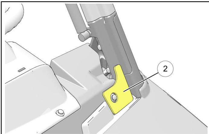
17. Close windshield and lock handle into base (5). Ensure windshield seal is adequately compressed and windshield opens/closes properly. Adjust as required.
