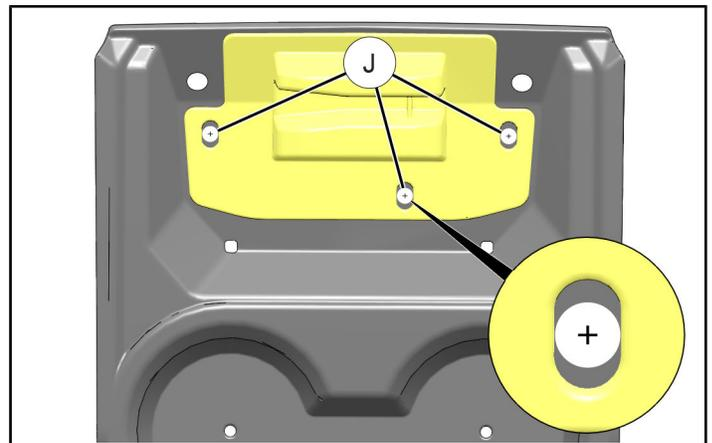
14. Drill 9/32 inch (7 mm) holes through cupholder at marked locations (J).
