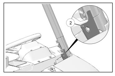
3. Open four clamps (A), position lower edge of windshield (1) against dash panel, then lock clamps to A-pillars.
