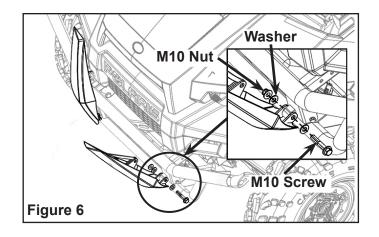
Install LH side front guard assembly by aligning lower cast mount to the outer cast pivot. Loosely install two M10 screws at lower weld bracket. Figure 7.
