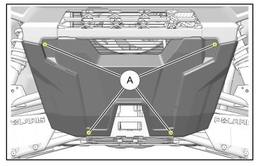
3. Reinstall and tighten upper two screws (A).
