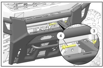
Secure bumper to chassis at lower mounting locations using two each NEW screws ② and nuts
