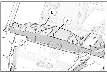
ii. Using fingers, remove center storage box © by pressing top edge of box down, disengaging box locking tabs from main dash panel as shown. Tip box out of dash and remove.
