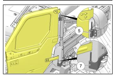
b. Close and push door inwards while centering door in ROPS/chassis opening, then tighten all screws ④.
