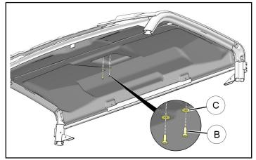
d. Carefully pull LH and RH edges of liner from between ROPS and roof seal, then remove rear edge of liner from roof support channel ().
