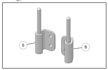
c. Install upper LH chassis-side hinge (5) using two screws (4) and nut plate (6). Partially tighten screws (but still loose enough to allow hinge movement).
