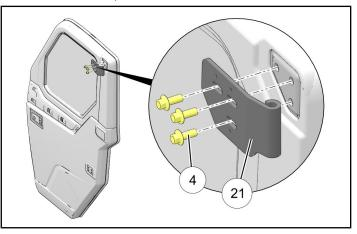
c. Install lower door-side hinge <sup>(2)</sup> to LH door <sup>(1)</sup> using four screws <sup>(4)</sup>. Partially tighten screws (but still loose enough to allow hinge movement).
