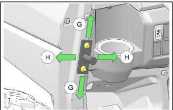
c. Torque striker screws ④ to specification.
