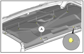
c. If overhead light is installed against liner, remove it. Otherwise, remove two each screws
