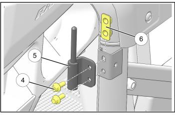
d. Install lower LH chassis-side hinge ⑦ using two screws ④. Tighten screws.
