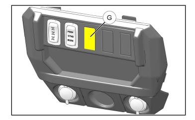
e. Install switch ② in control panel opening.
