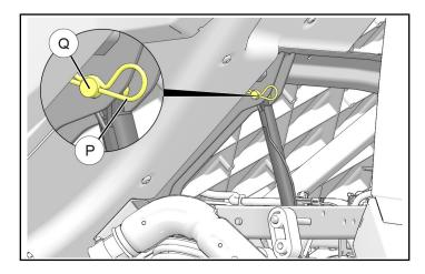
10. Install box lift actuator ① to chassis mounting bracket using retained clevis pin @ and hairpin clip
