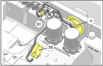
b. Drill out one accessory plug (1/4 inch / 6 mm) on under-hood liner, forward of air intake ducts, then install relay/fuse block 3B using attached fir tree clip.
