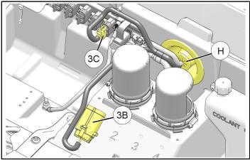
Drill out one accessory plug (1/4 inch / 6 mm) on under-hood liner, forward of air intake ducts, then install relay/fuse block 3B using attached fir tree clip.
