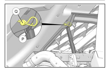
Install box lift actuator ① to chassis mounting bracket using retained clevis pin ② and hairpin clip
