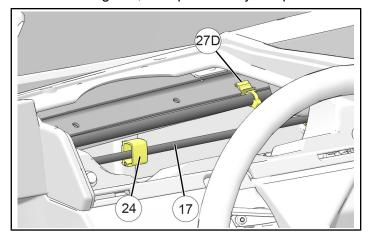
c. Continue routing A-pillar harness ② and washer bottle hose ① towards LH A-pillar. Reaching through LH side of instrument panel cutout, secure A-pillar harness to front dash bracket using two remaining edge clips 27D.
