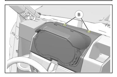
3. Install windshield wiper housing assembly.
