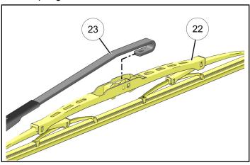
g. Orient wiper blade/arm assembly parallel to top of windshield, then install to motor shaft ①.
