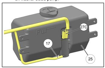
d. Join harness connector 27C to mating connector on washer bottle pump.
